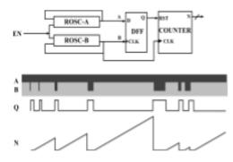
Fig.1: Architecture of single phase BFD-TRNG.
